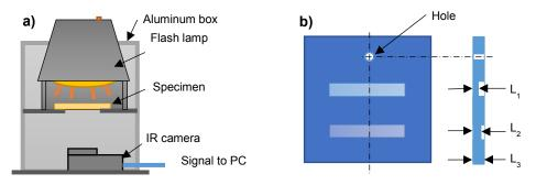
Fig. 1: a)Schematic of experimental apparatus used for the measurement of thermal diffusivity via the flash method; b) schematic of specimen object of measurements
