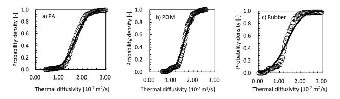
Fig. 3: Comparison of results distribution with Gaussian type distribution for a) PA, b) POM and c) rubber
