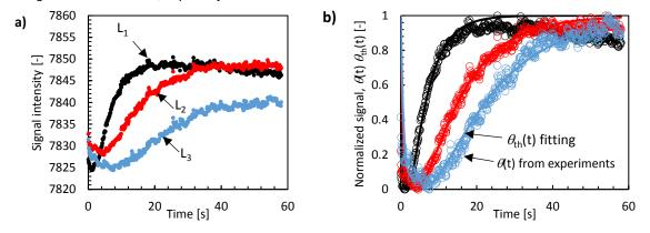
**Fig. 2:** a) Typical results of raw data of IR signal intensity measured for a PA specimen in correspondence of thickness L<sub>1</sub>, L<sub>2</sub> and L<sub>3</sub>; b) normalization of raw data and comparison with fitting curve
