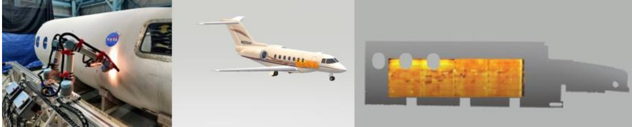
Fig. 2: Dual collaborative robot thermal line scan inspection of aircraft fuselage.
